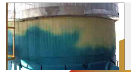
CT-IP180 is a one time warning system. The colour change is permanent.
